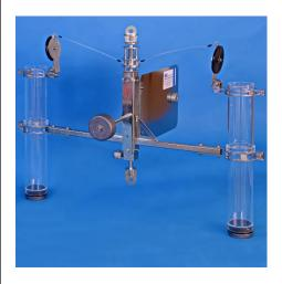
2 sample tubes, steering fin and a balance arm
